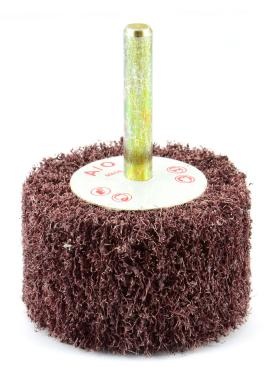
ARC Abrasives' Mounted and Unmounted Flap Wheels are versatile tools ideal for light grinding, blending, deburring, and finishing applications on a wide variety of metals. The radial flap design ensures a continuous supply of fresh abrasive grains, delivering consistent cutting action and a smooth finish. These flap wheels conform to different geometries, making them perfect for both flat and contoured surfaces.
