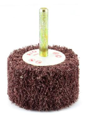
ARC Abrasives' Mounted and Unmounted Flap Wheels are versatile tools ideal for light grinding, blending, deburring, and finishing applications on a wide variety of metals. The radial flap design ensures a continuous supply of fresh abrasive grains, delivering consistent cutting action and a smooth finish. These flap wheels conform to different geometries, making them perfect for both flat and contoured surfaces.
