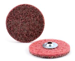
ARC Abrasives' Z-WEB Surface Conditioning Quick-Lok Discs offer an advanced solution for efficient surface conditioning and cleaning & finishing tasks. Available with three different styles of self-centering locking mechanisms, these discs ensure fast and precise disc changes, reducing downtime and enhancing productivity. Their open nylon web structure minimizes loading and adapts to the workpiece shape, while the surface conditioning discs feature reinforced backing for added durability.
