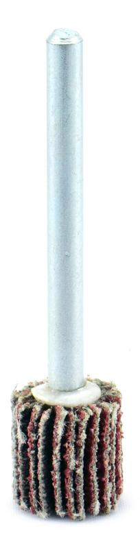
ARC Abrasives' Mounted and Unmounted Flap Wheels are versatile tools ideal for light grinding, blending, deburring, and finishing applications on a wide variety of metals. The radial flap design ensures a continuous supply of fresh abrasive grains, delivering consistent cutting action and a smooth finish. These flap wheels conform to different geometries, making them perfect for both flat and contoured surfaces.
