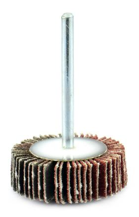
ARC Abrasives' Mounted and Unmounted Flap Wheels are versatile tools ideal for light grinding, blending, deburring, and finishing applications on a wide variety of metals. The radial flap design ensures a continuous supply of fresh abrasive grains, delivering consistent cutting action and a smooth finish. These flap wheels conform to different geometries, making them perfect for both flat and contoured surfaces.
