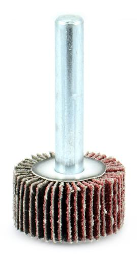
ARC Abrasives' Mounted and Unmounted Flap Wheels are versatile tools ideal for light grinding, blending, deburring, and finishing applications on a wide variety of metals. The radial flap design ensures a continuous supply of fresh abrasive grains, delivering consistent cutting action and a smooth finish. These flap wheels conform to different geometries, making them perfect for both flat and contoured surfaces.
