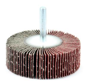
ARC Abrasives' Mounted and Unmounted Flap Wheels are versatile tools ideal for light grinding, blending, deburring, and finishing applications on a wide variety of metals. The radial flap design ensures a continuous supply of fresh abrasive grains, delivering consistent cutting action and a smooth finish. These flap wheels conform to different geometries, making them perfect for both flat and contoured surfaces.
